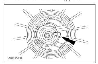
53. **CAUTION:** If the strut is installed incorrectly, transmission damage will occur.
